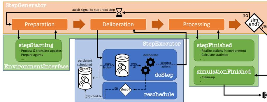
Fig. 4: The StepGenerator calls the appropriate methods on the StepExecutor and registered EnvironmentInterfaces to initiate the *preparation*, *deliberation*, and *processing* phases in each time step.
