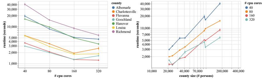
Fig. 6: The mean runtime of PanSim+Sim-2APL simulations for seven counties of the state of Virginia compared with (a) the number of cores, and (b) the number of agents.
